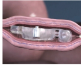
B: Outer shell dissolves and the balloon starts to inflate as the reaction begins.
