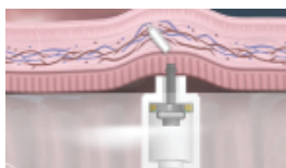
C: Pressure in the balloon pushes the dissolving microneedle into the intestinal wall.
